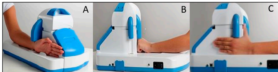
Figure 1. BAUSport™ Sonic Bone protocol measurement—(A) 1st hand measurements position—wrist; (B) 2nd hand measurements position—phalanges; (C) 3rd hand measurements position—metacarpals ( https://sonicbonemedical.com/product/ , accessed on 20 February 2026).
